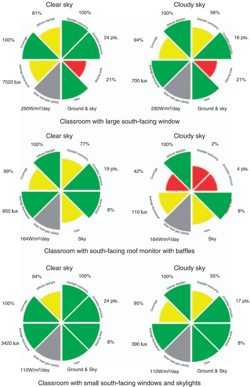
**Figure 3** Daylighting dashboards for the three classroom designs considered in the example (from Leslie *et al.*<sup>19</sup>). Note: in the online version of this paper white is denoted by red, grey by yellow, and black by green. The solar heat gain is denoted by hatched gray
