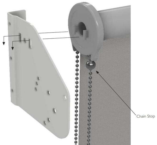
Add ball stop to front chain when shade is in the correct closed (down) position – add ball stop to rear chain when shade is in the correct open (up) position.
