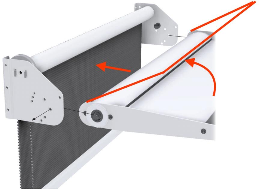
With the lightshelf held at an angle compress the spring-loaded pin-ends and slide it back into the “hockey stick” slots until it snaps in – slide the lightshelf back until the pin-ends seat into the end of the slot.
