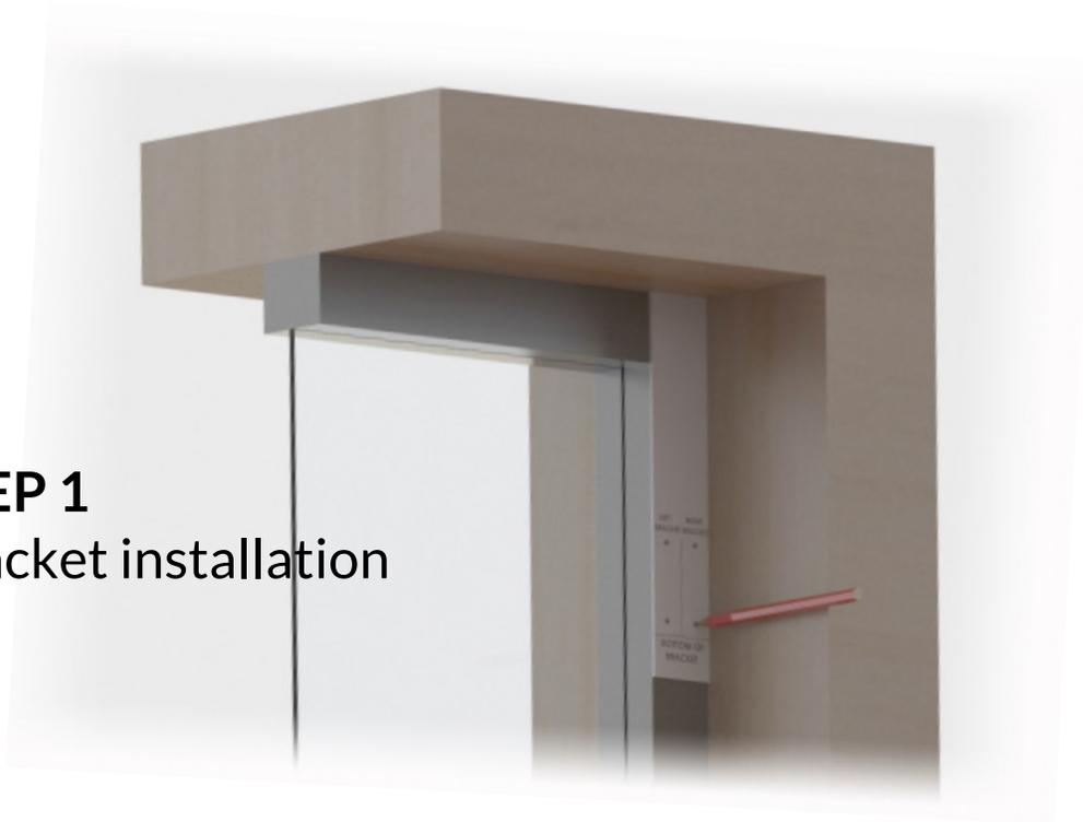
Using the template provided hold against the window head and mark the location of the mounting screws. Use against window frame for front mount and against jamb for side mount. If no template is available mark the bottom of the bracket using the lightshelf size as a guide (mark 16" down for S1600 lightshelf, 18" for S1800 etc.)
