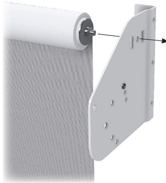
With pin-end compressed slide (walrus) teeth into slotted openings and pull down until the clutch is seated firmly in the slots.
