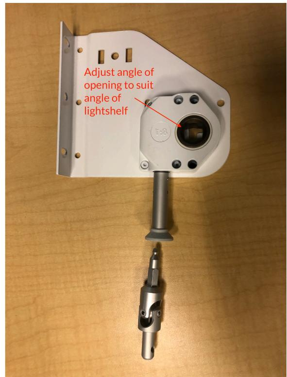
Insert the square drive pin into the worm drive first (having roughly matched the angle of the square opening to the angle of the lightshelf). Compress the heavy-duty pin-end and slide it back into the “hockey stick” slot until it snaps in – slide the lightshelf back until the pin-end seats into the end of the slot. Finally, insert a crank into worm drive and test for free rotation and proper horizontal position against rubber stop.
