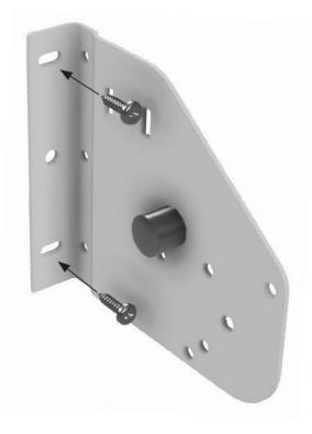
Attach mounting brackets with the appropriate screws (provided). Note that one bracket will have a rubber stop the other a worm drive attached.
