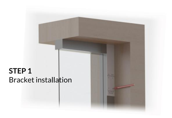
Using the template provided hold against the window head and mark the location of the mounting screws. Use against window frame for front mount and against jamb for side mount. If no template is available mark the bottom of the bracket using the lightshelf size as a guide (mark 16" down for \$1600 lightshelf, 18" for \$1800 etc.)
