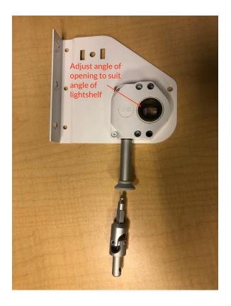
Insert the square drive pin into the worm drive first (having roughly matched the angle of the square opening to the angle of the lightshelf). Compress the heavy-duty pin-end and slide it back into the "hockey stick" slot until it snaps in – slide the lightshelf back until the pin-end seats into the end of the slot. Finally, insert a crank into worm drive and test for free rotation and proper horizontal position against rubber stop.
