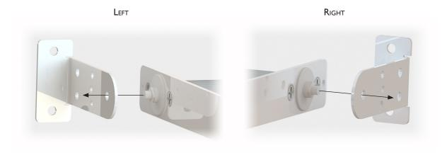
NOTE: Bracket on Worm Gear side to be installed with flange away from jamb - Bracket on Pin End side to be installed normally, flange to jamb
