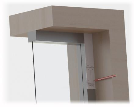
NOTE: Template should be positioned on the jamb for inside mount
